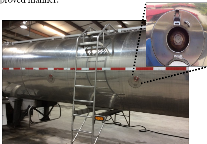
Milk Tanker Truck w/QMI Insulated Fitting and Aseptic Sampling Port Installed on the Side
