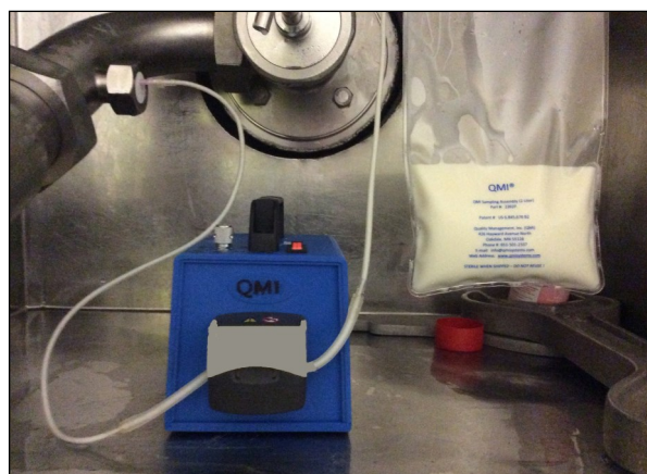
QMI Portable Peristaltic Pump w/QMI Fitting & Composite Sampling Bag in Rear of Truck
