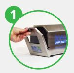
Rotate spring loaded door closure screw to the left. Unscrew lid. Pull lid down.
