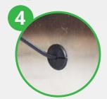
Slide black grommet over electrical cord. Grommet needs to have slit in it.
