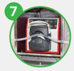
Place silicone section of the line set into clamshell, close clamshell over tubing. Push pump securely to the back.
