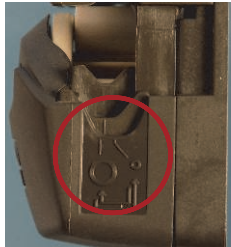
Outer position, for large tubing
