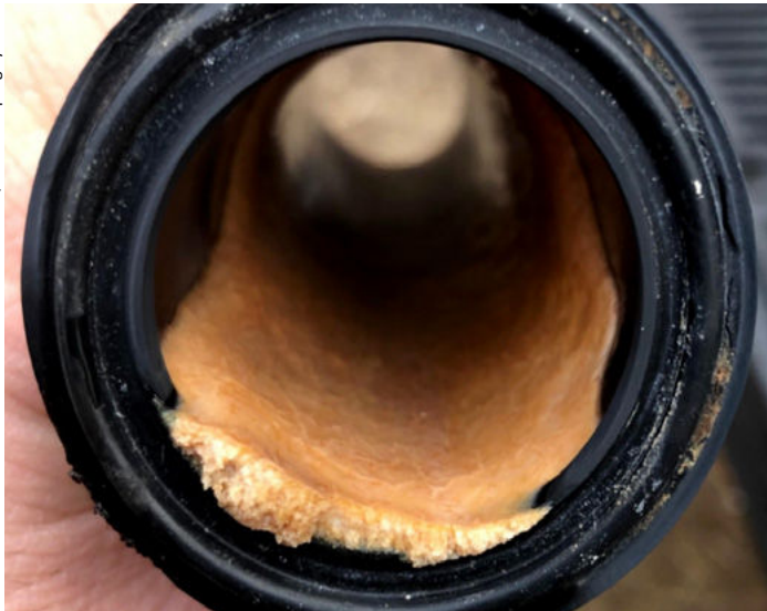
Bacterial biofilms attach to environmental surfaces and grow into dense mats that persistently contaminate raw or pasteurized products. Once established, biofilms are difficult to eradicate. Continual process monitoring is critical to isolate biofilms in the early stages of development before they can become fully established.
