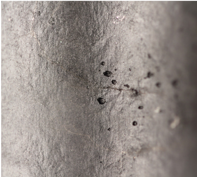
Corrosion, cracking, and pitting in 316 stainless steel pipe that has been etched with acid. Pits, cracks, and fissures may become attachment sites for biofilms.
