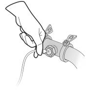
**NOTE:** The nut may need to be re-tightened periodically due to vibration and cleaning cycles.
