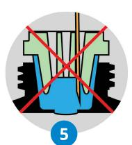
Do not spin or twist on the way through, as you could core the rubber.
