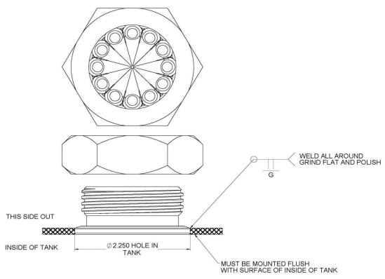
NOTE: THIS DIAGRAM DOES NOT APPLY TO ELLIPTICAL TANK DOORS OR TO MUELLER TANK DOORS. FOR THOSE INSTALLATIONS, CALL QUALITRU FOR INSTRUCTIONS.
