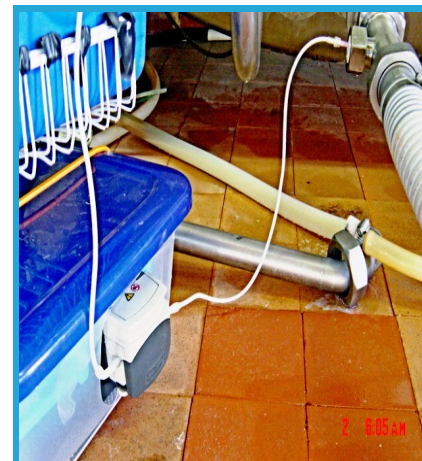
Peristaltic Pump and QMI Sampler used to obtain sampling data for NCIMS approval
