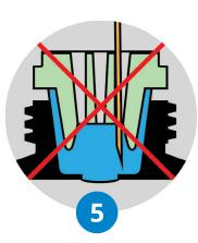
Do not spin or twist on the way through, as you could core the rubber.
