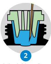
Face the bevel of the needle outward, or toward the outer ring.
